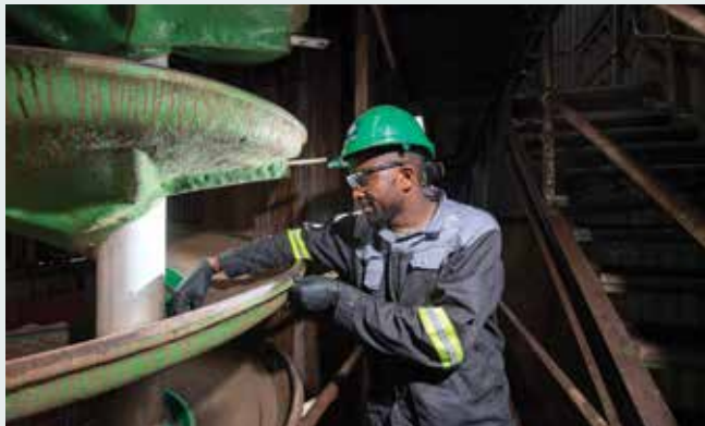
Multotec UX7 spiral testing was conducted on chrome, manganese and iron ore but can also be applied in copper, platinum and other metals.
