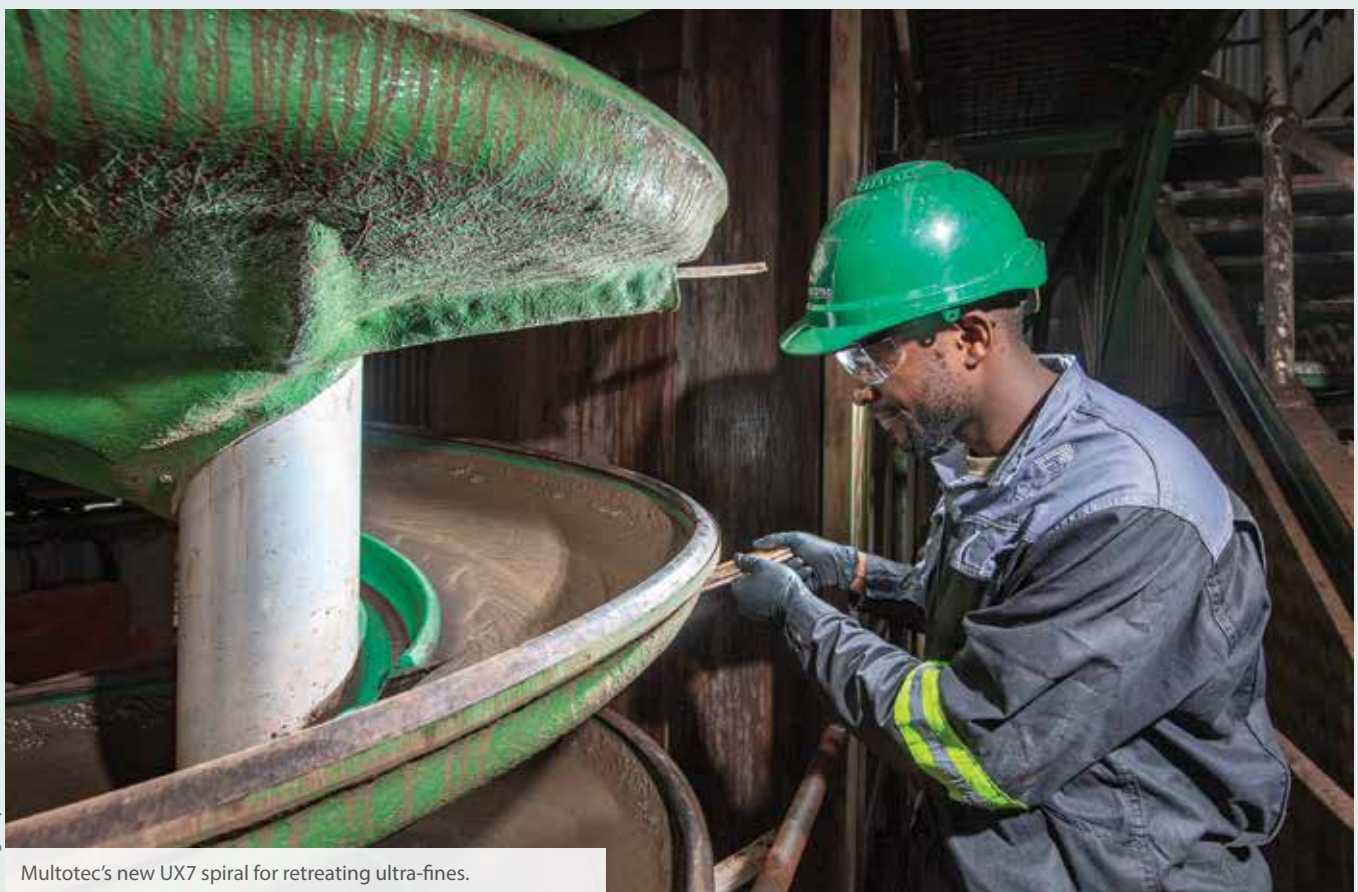
Multotec UX7 spiral testing was conducted on chrome, manganese and iron ore but can also be applied in copper, platinum and other metals.
