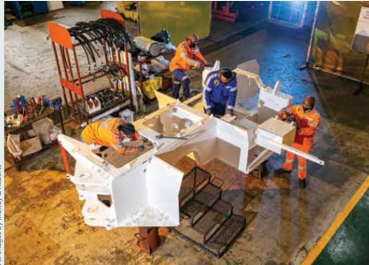
Fitting of engine frame and components before assembly commences on a 5.5 t load-haul-dumper.
