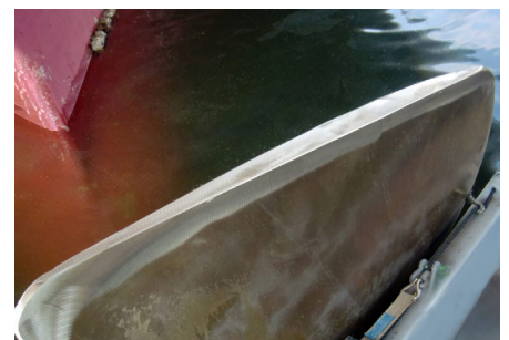
ONE OF THE PROPELLER BLADES OF A BULKER WAS MISSING PARTS. CAREFUL RESTORATION ENSURED IT WAS BACK TO WORKING ORDER
